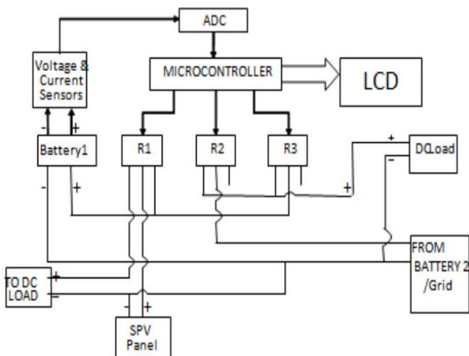
Fig-2: Block diagram of proposed net metering
