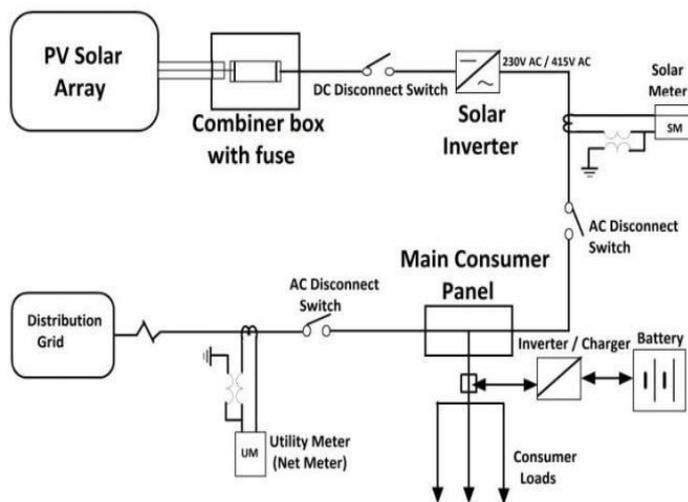
Fig 1: Net Metering arrangements
