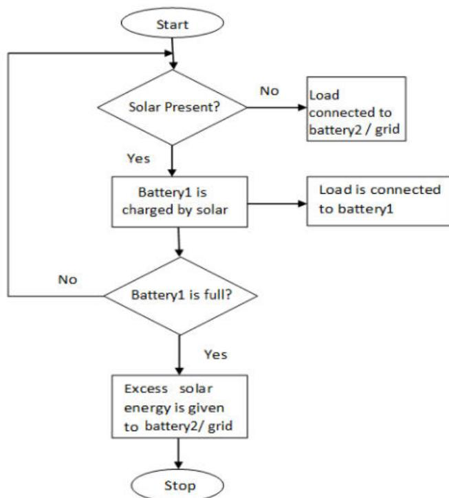
Fig 3: Flowchart of proposed net-metering concept
